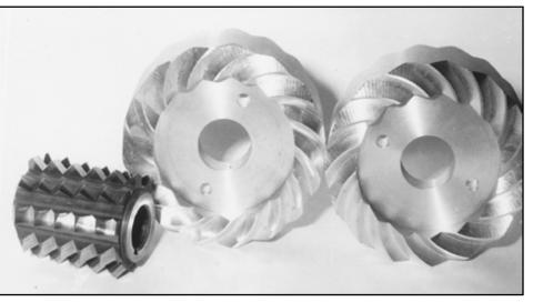
Figure 6: Experimental involute spiral face coupling mating flanges and hob (the same hob was used to machine both right and left hand spiral face gears)
